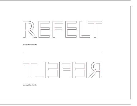
1.4 Combining multiple shapes as a puzzle When multiple shapes and / or colors are combined as one single layer puzzle, the shapes must connect exactly in de cutting drawing. The knives that are used for cutting PET Felt are very thin, therefore there is no cutting loss. All shapes in a specific color need to be drawn on the panel dimensions and submitted as separate files.
