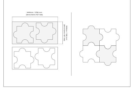
**1.5 Part spacing and margins: Nesting** If you require multiple shapes being cut out of one PET Felt panel these can be positioned with at least 6mm in between these parts.
