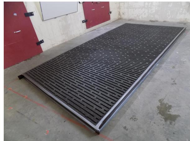
Absorb, versie 5.8.4 mode 7, PM: MH, file: a3229#1-36 F#:407-442 A#:443 T<sub>1</sub> = 15,8 °C T<sub>2</sub> = 16,0 °C p<sub>1</sub> = 100,0 kPa p<sub>2</sub> = 100,3 kPa h<sub>1</sub> = 49,7 % h<sub>2</sub> = 57,4 %volume reverberation room: 214 m<sup>3</sup>surface area sample: 11,9 m<sup>2</sup>
